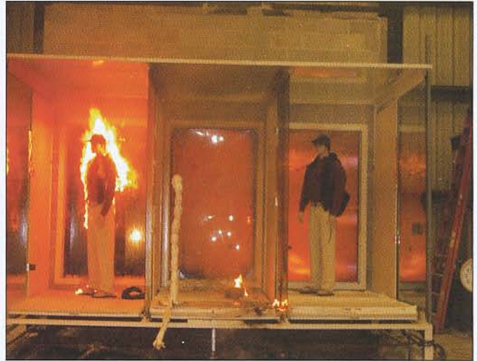
The results of testing based on the setup shown on page 56. At left, the mannequin behind the wired glass spontaneously ignites at approximately nine minutes. On the right, the mannequin behind the ceramic glass ignites at around the 11-minute mark.
