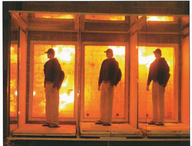
Glazing samples (from left to right: ceramic, wired, and heat reflective specialty tempered) in front of the test furnace.
