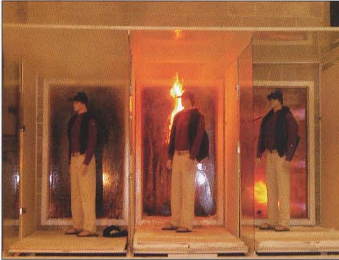
The results of testing based on the setup shown on page 56. At left, the mannequin behind the wired glass spontaneously ignites at approximately nine minutes. On the right, the mannequin behind the ceramic glass ignites at around the 11-minute mark.
