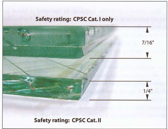
A visual comparison of two safety-rated wired glass products.
